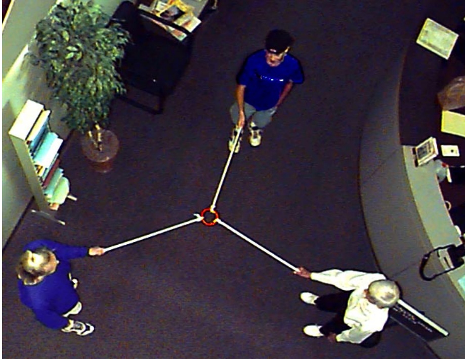
Figure 13. Three people pull ropes tied to a central ring. The ring moves not toward any single puller but in the direction of the vector sum — the resultant of the three forces.
